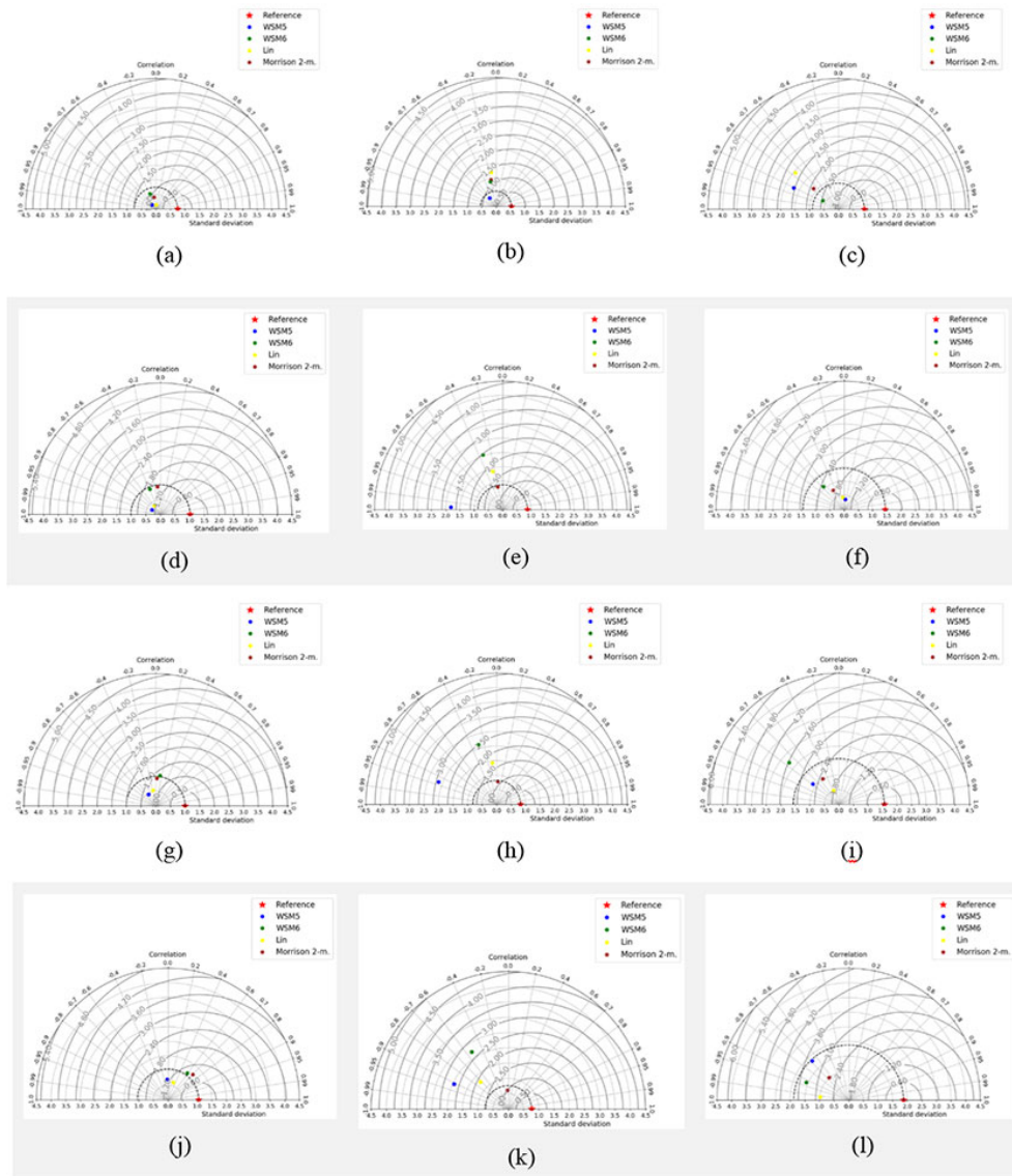
Figure 11. Taylor diagrams for rainy season LLWS speed forecast, panel from left to right pre-, in- and after- storm statics at (a,b,c) 0-360 ft (d,e,f) 0-1060 ft (g,h,i) 0-1770 ft (j,k,l) 0-2500 ft.
